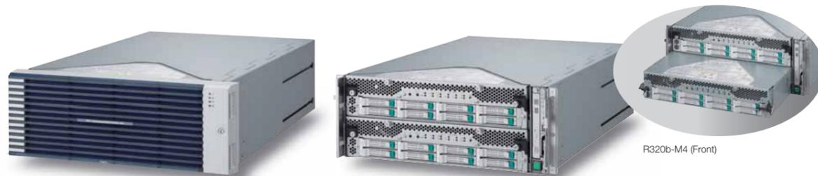
Fully redundant by dual modular architecture
