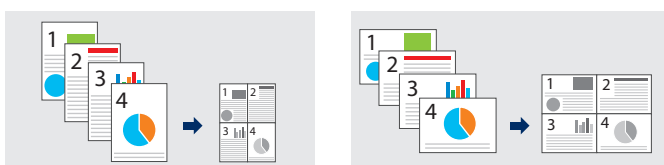
4IN1 : Copies four pages on a sheet of paper in portrait or landscape orientation.
